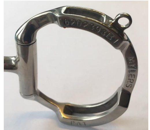
The 2016 Eggbutt with Hooks. The rein hook has been lengthened to prevent the rein kinking and the hole has been replaced by a loop
