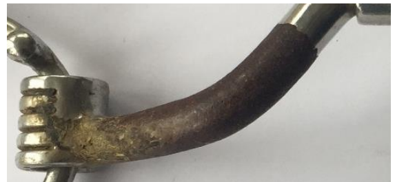
Clean the bit after each use to ensure the metal corrodes evenly. NOT like this owner!
